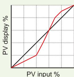
Linearisation of signals with square characteristic such as flow rate
