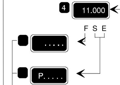
Function 4 has been selected. It consists of three parameters.. The first parameter is indicated without a decimal point in the function display. It has a floating point. After confirming the last digit, the decimal point's position may be changed through Scroll. Pressing Enter will confirm it's position.
