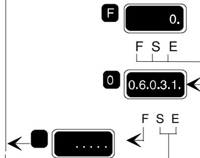
The previously set parameter is displayed blinking. The digit may be edited by pressing Scroll and confirmed by pressing Enter. By pressing F input is interrupted and the edited digit is not stored in the EEPROM. The parameter remains unchanged.
