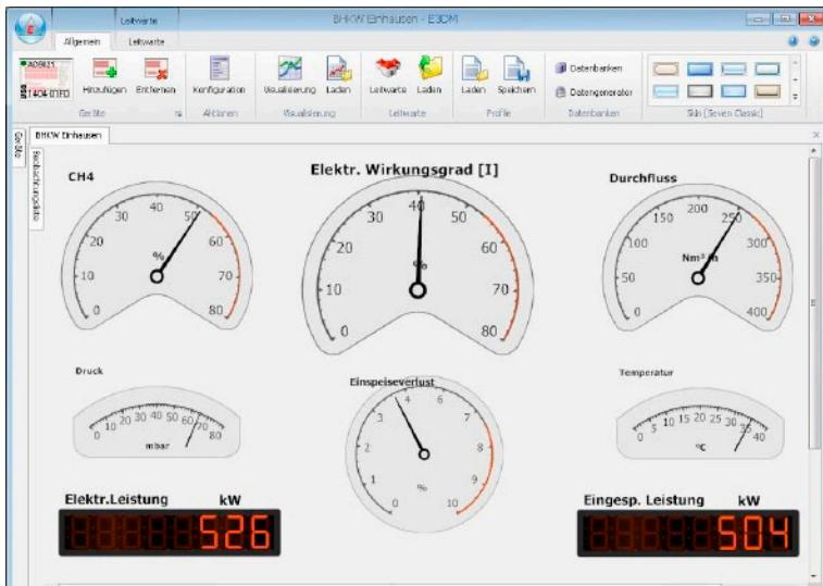
In the master display the actual measured values are mapped. The amount of the displayed values and the graphical illustration can be adjusted individually.
