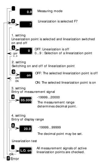
If the measurement value should not be linear to the measurement range, the values may be adjusted accordingly. Up to 10 signals with appropriate display values may be set. They are called linearization points and are arranged from 0 to 9. Function 7 - linearization is performed <u>after</u> measurement range setting in function 1. The signals lie within initial and end of the measurement range as scaled under function F1.
