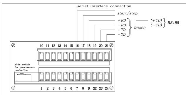
Terminals 18-21 are used for either the serial interface or the analogue output.
