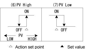
\* ON/OFF in the diagrams indicate operation mode. EVENT/DO output conforms to the setting (OPEN/CLOSE) of output characteristics.
