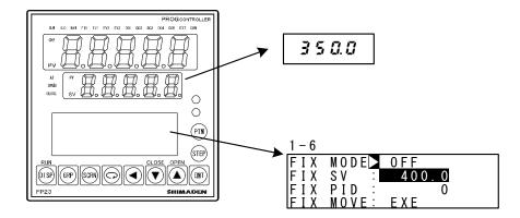
The white-inverted section indicates limiter over.
