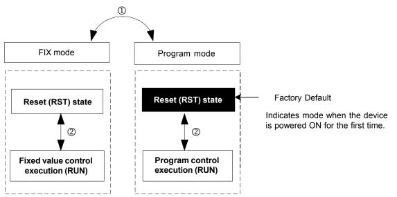
The control mode is switched by the FIX mode ON/OFF settings in the FIX MODE screen (No.1 to 6). The Mode switches to the FIX (fixed value) mode when ON is set, and to the Program mode when OFF is set.
