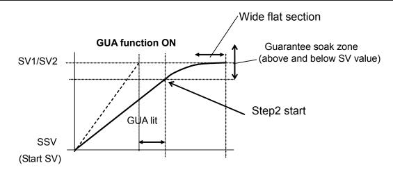
When the deviation between the step SV and PV of the flat step does not enter the guarantee soak zone when the ramp step switches to the flat step, the program does not move to the next step, and program execution stands by until this region is reached or the GUA time ends.
