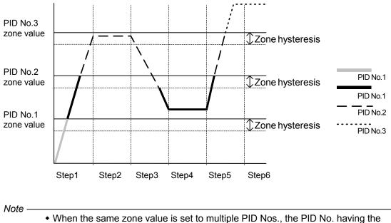
When the same zone value is set to multiple PID Nos., the PID No. having the smallest No. is executed.
