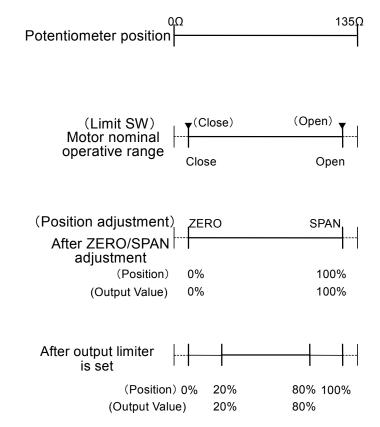
\* Operative range by the output limiter (for details, refer to "11-7" Output Limit Value (OUT1L to OUT1H)) at lower limit = 20% and upper limit = 80%
