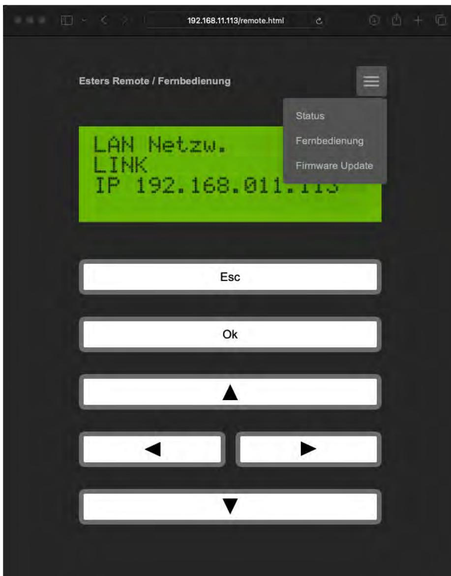
**Figure 42: Web page for remote control of the device II**
