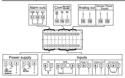
Note Do not connect other than the specified input type to terminal.
